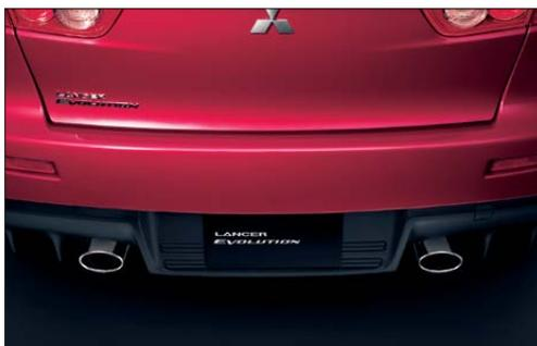
The rear-oriented exhaust layout makes the exhaust piping shorter and more direct. In addition, output losses are reduced by the larger intake port, increased main muffler capacity and large-diameter dual tail pipe arrangement. The space saved by the new layout of the intake and rear exhaust, in addition to moving the battery to the trunk space, has made it possible to achieve a smoother airflow through the air filter and intercooler, with lower aerodynamic drag.
