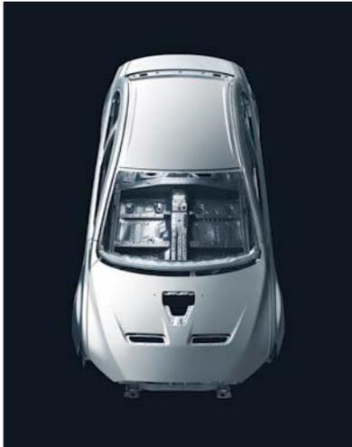
To reduce the overall vehicle weight, the roof panel, engine hood, front fenders and front and rear bumper beams have all been made with lightweight aluminum. In addition to increasing body rigidity while lowering weight, weight reduction has been focused on the upper part of the vehicle to improve control and performance.
